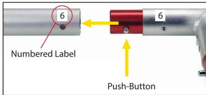
Connections are made by holding the button down and sliding the red tube into opposing tube until button locks into the hole of the opposing tube. To disassemble, push button and pull or twist extrusions apart.
